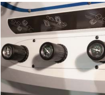
Three pressure regulators
